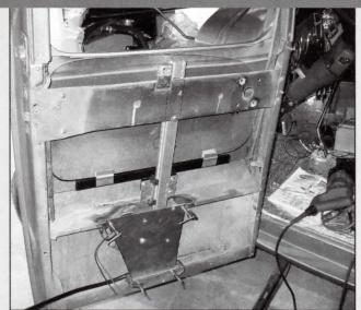
Now Bob checks the alignment with the window in place and the tract secured with clamps. As long as the glass moves freely at this point, go ahead and tack the mount to the door. It's a good idea to recheck the window's movement one more time before welding the mount completely.
