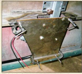
With the track and motor mounted to the mounting plates, the up and down action of the glass should be tested at this time to insure no binding. This is very important, as you wouldn't want to have to cut the brace out before you know it will even work in that position. Clamping in place like this will save some frustration for sure.
