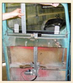
With the notch taken out of the brace, the track slides into place with the necessary angle to lift and lower the glass without any bind. This is also the time to cut off the unnecessary length of vertical track. The track is engineered extra long for a custom fit in many different applications.
