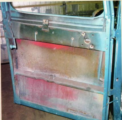
Like we said earlier, this particular door panel unscrews completely, giving us great visibility and accessibility to the inner part of the door. While many trucks are set up like this, most cars are not, usually necessitating some cutting of the inner door structure.
