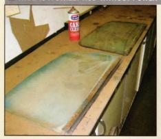
Everything will need to be taken out of the door and set aside for now, even the inner door handle and mechanism. This is the best time to thoroughly clean the glass and to remove the old channel at the bottom edge of the glass.
