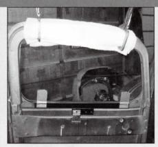
While the brackets are being tacked into place, Bob uses a couple of vise-grips and a towel to hold the glass in the closed position. There is another bracket that will need to be attached at the top of the track.
