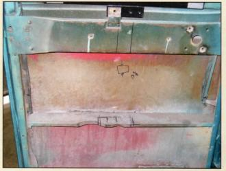
A preliminary fit showed a problem with the factory brace running horizontally through the middle of the door. This will be some of the minor custom work necessary for a correct installation.
